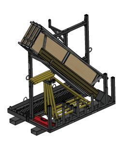
6) Place cross braces in front of the side toeboards and on top of the cat-a-corner brace. Slide braces into the bottom rack pocket.
