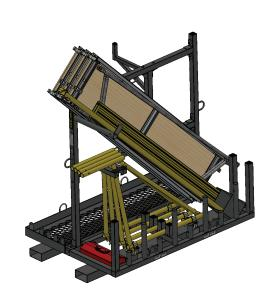
7) Place casters in front of the outriggers. Insert the stem end into the vertical tube. Secure each in place with a snap pin.
