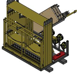
11) Use **10' strap** - attach to ring **A** and wrap across the frames and end guard panels, and attach to ring **B**. Tighten strap.
