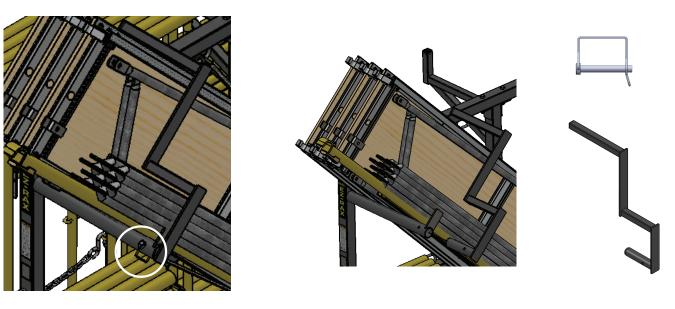
5) Remove snap pin from the outrigger latch and rotate open. Place snap pin back into support bar, so as not to misplace.
